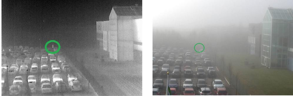
Figure 3 Image from a thermal camera (left) and a visual camera (right) on a misty day
