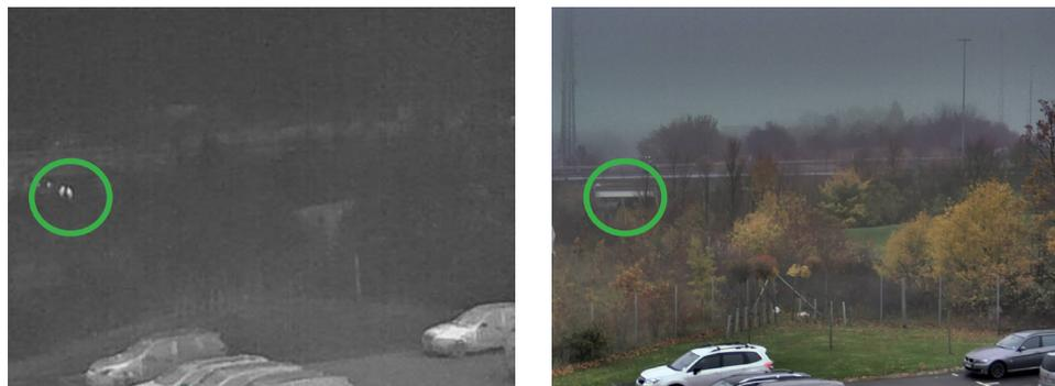
*Figure 5. Images of persons taken with a thermal camera (left) and a visual camera (right) on a rainy day*
