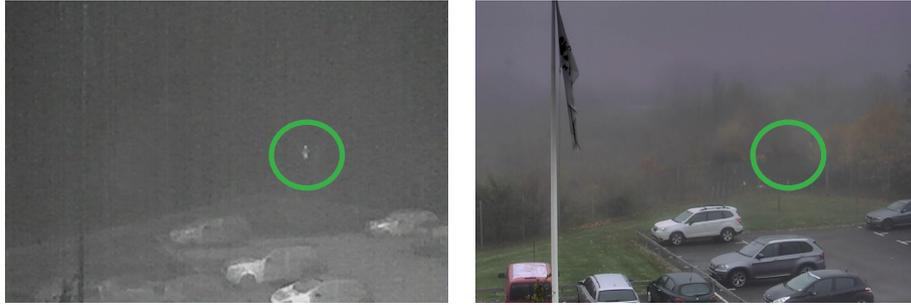
Figure 4. Images of a person taken with a thermal camera (left) and a visual camera (right) on a foggy day
